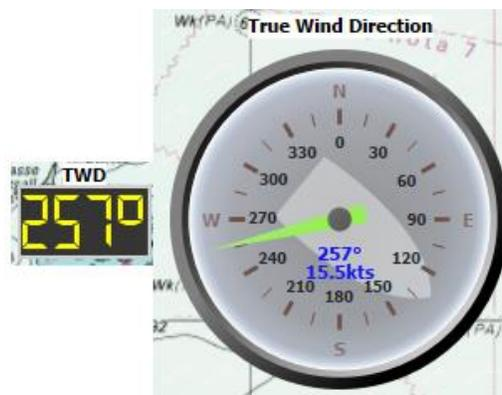
This instrument shows True Wind Direction. If NMEA data do not provide it and if it is possible, qtVIm will calculate it based on COG, SOG and apparent wind data. The arrow's color changes with wind speed, and boat orientation is drawn on background.
