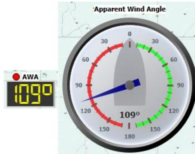
This instrument displays Apparent Wind Angle. If NMEA data do not provide it and if it is possible, qtVIm will calculate it based on COG, SOG and real wind data.
