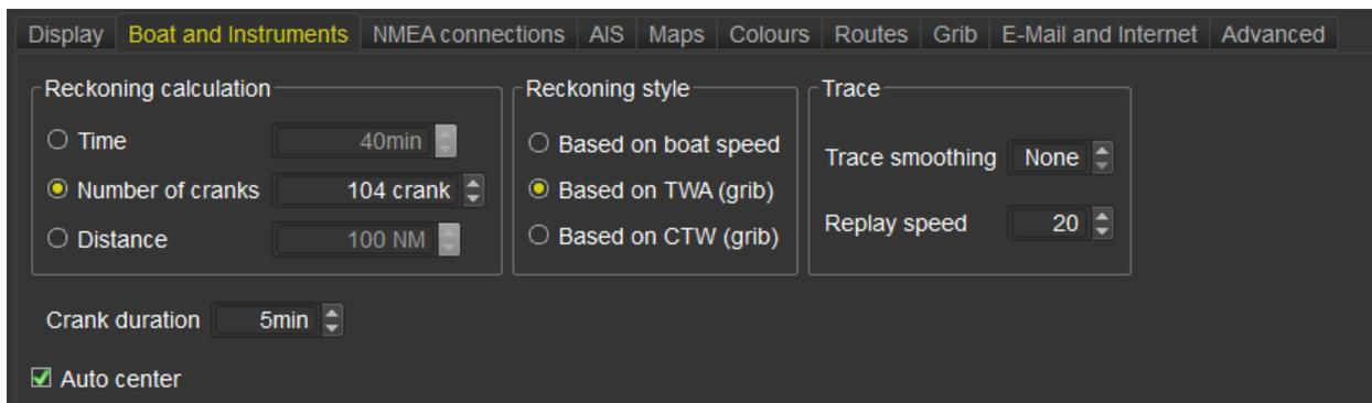
Apart from various reckoning and trace options, you can specify here what Crank duration qtVIm will use. This is the internal step qtVIm is using for all calculations. A small value gives more precise results, but will be costlier in CPU, memory and computation times.
