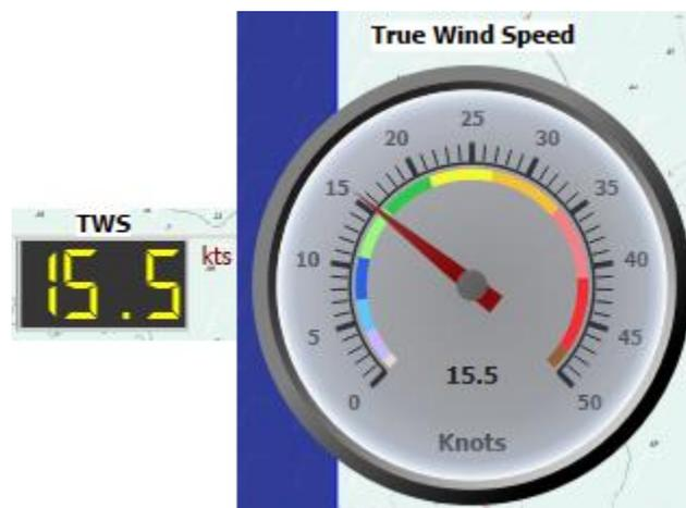
This instrument displays True Wind Speed. If NMEA data do not provide it and if it is possible, qtVIm will calculate it based on COG, SOG and apparent wind data.
