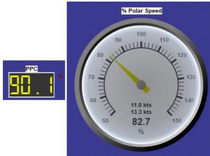
This instrument shows the difference between actual speed and theoretical polar speed, as a percentage and as values. It is also possible to send this data through the NMEA output port in order to display it on NKE or Raymarine instruments.
