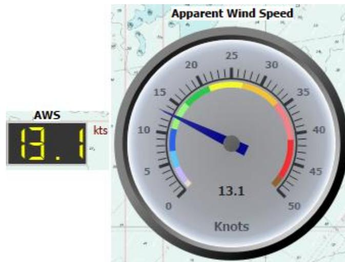
This instrument displays Apparent Wind Speed. If NMEA data do not provide it and if it is possible, qtVIm will calculate it based on COG, SOG and real wind data.
