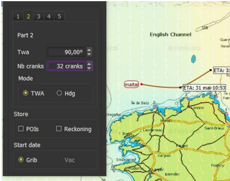
This function calculates the boat's position based on polar and grib Winds data. Five legs can be defined, either in fix TWA or fix heading mode. Penalties for tack/gybes, and waves parameters are **not** taken in account.
