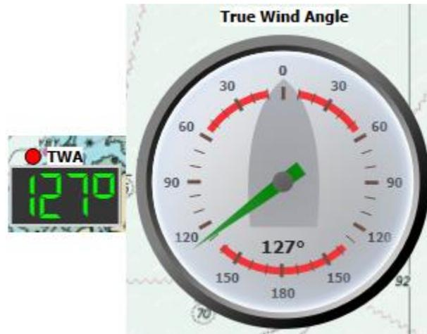
This instrument shows True Wind Angle. If NMEA data do not provide it and if it is possible, qtVIm will calculate it based on COG, SOG and apparent wind data. The value and the arrow is green when TWA is inside the polar VMG limits, red otherwise. The digital display also shows a red or green dot, depending on the tack. The red parts on the dial represent the polar VMG limits, and are recomputed dynamically.
