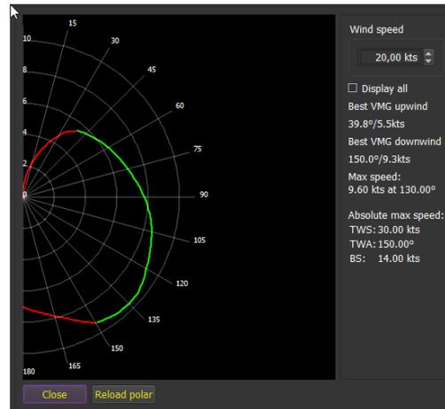
This dialog shows critical angles for the polar (best VMGs). Note that it is possible to modify the polar outside qtVlm in the same time. Just press "Reload polar" each time you save it.
