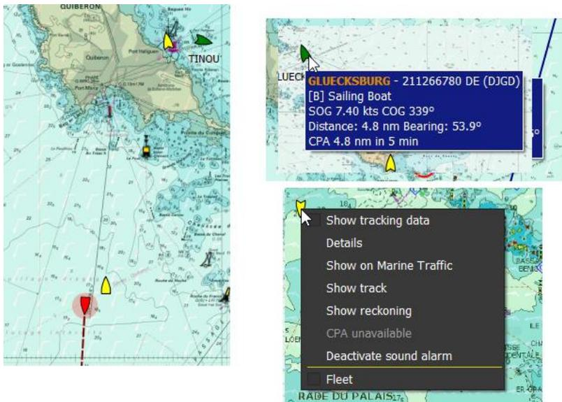
The screenshot shows a marine chart with a target 'GLUECKSBURG' highlighted. A tooltip displays the following information:
