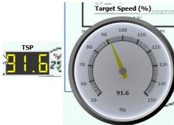
This instrument expresses the speed (SOG) in percentage of optimum speed as given by the polar to reach the WP. For instance, for a WP upwind, too much speed means you must luff a bit, while a percentage lower than 100% means you must ease a bit. This information is often more efficient than VMC for the helmsman.
