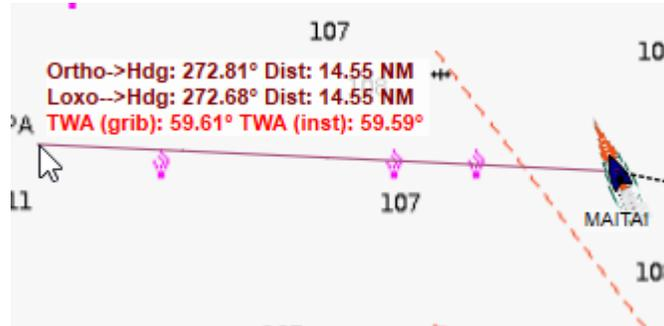
This function shows orthodromic and loxodromic lines with distances, angles, etc. It will turn red if crossing a land or a barrier. TWA data is also displayed, based on grib and instruments data.
