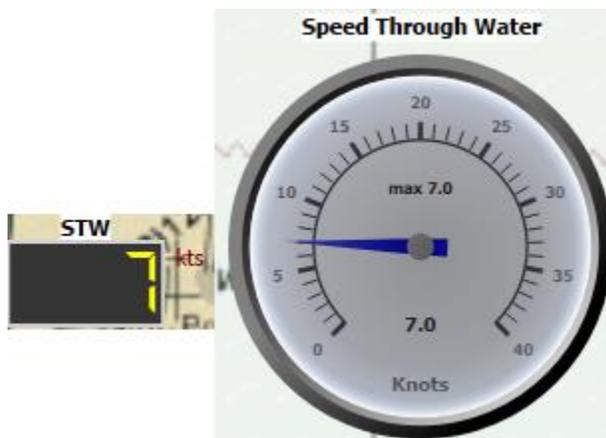
This instrument shows Speed Through Water. It is different from SOG in case of Currents, for instance. It also displays the maximum value measured.
