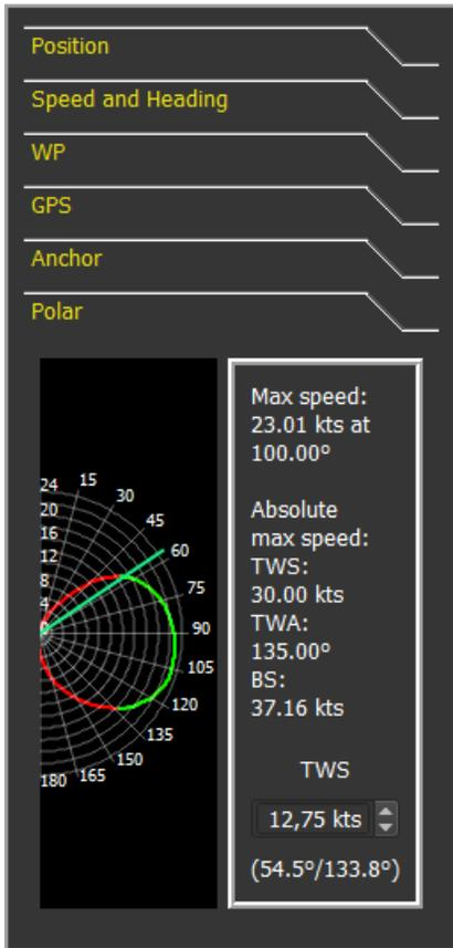
This tab shows boat's polar and display best wind angle upwind and downwind (left image).
