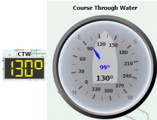
This instrument shows Course Through Water. It is different from COG in case of Currents, for instance. It also displays heading toward current waypoint (in blue).
